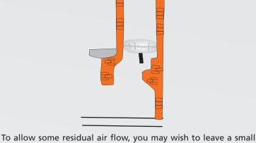
gap at one side of the balloon. For a video on how to use a chimney balloon, see
